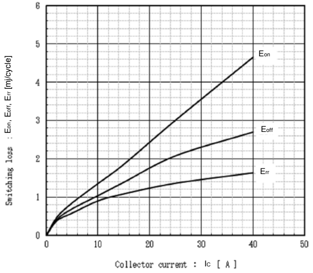
Switching Loss vs. Collector Current (typ.) V_{ce}=600V, V_{cc}=15V, T_j=125^{\circ}C
