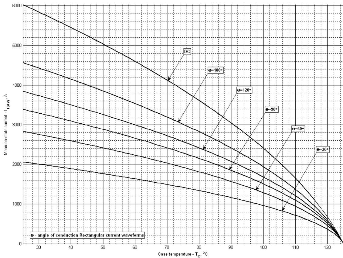
**Fig 12 – Maximum case temperature DSC (rectangular current waveforms)**
