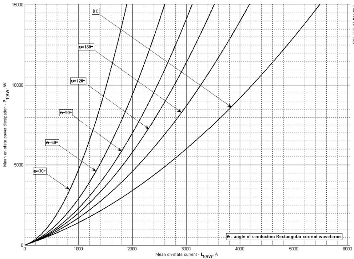
**Fig 10 – On-state power loss (rectangular current waveforms)**
