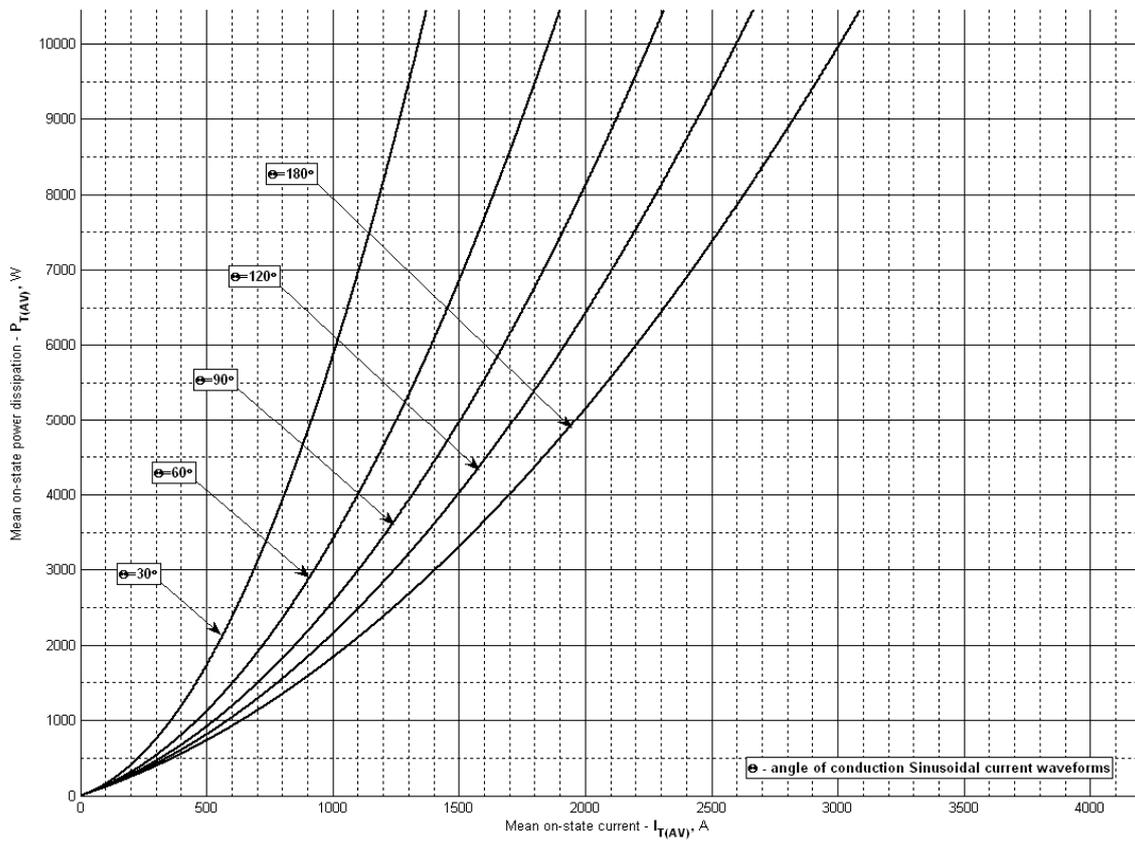
**Fig 9 – On-state power loss (sinusoidal current waveforms)**
