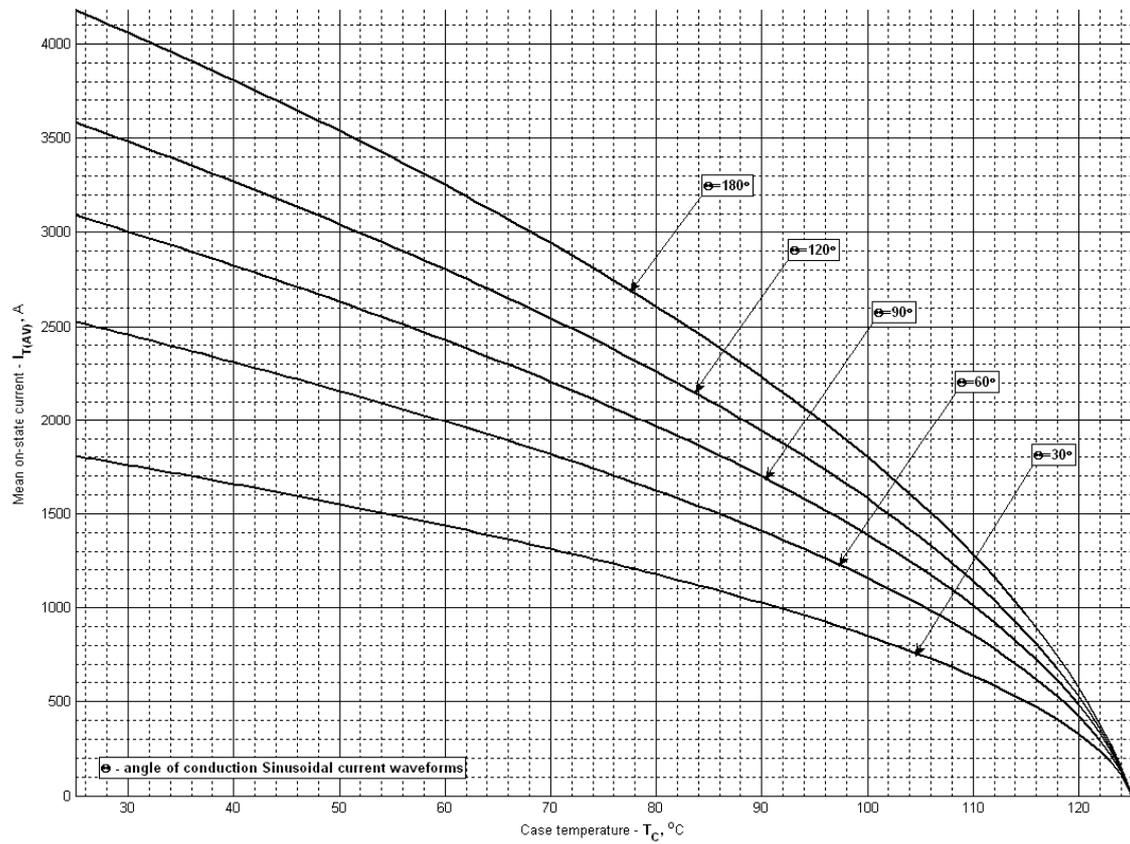
**Fig 11 – Maximum case temperature DSC (sinusoidal current waveforms)**
