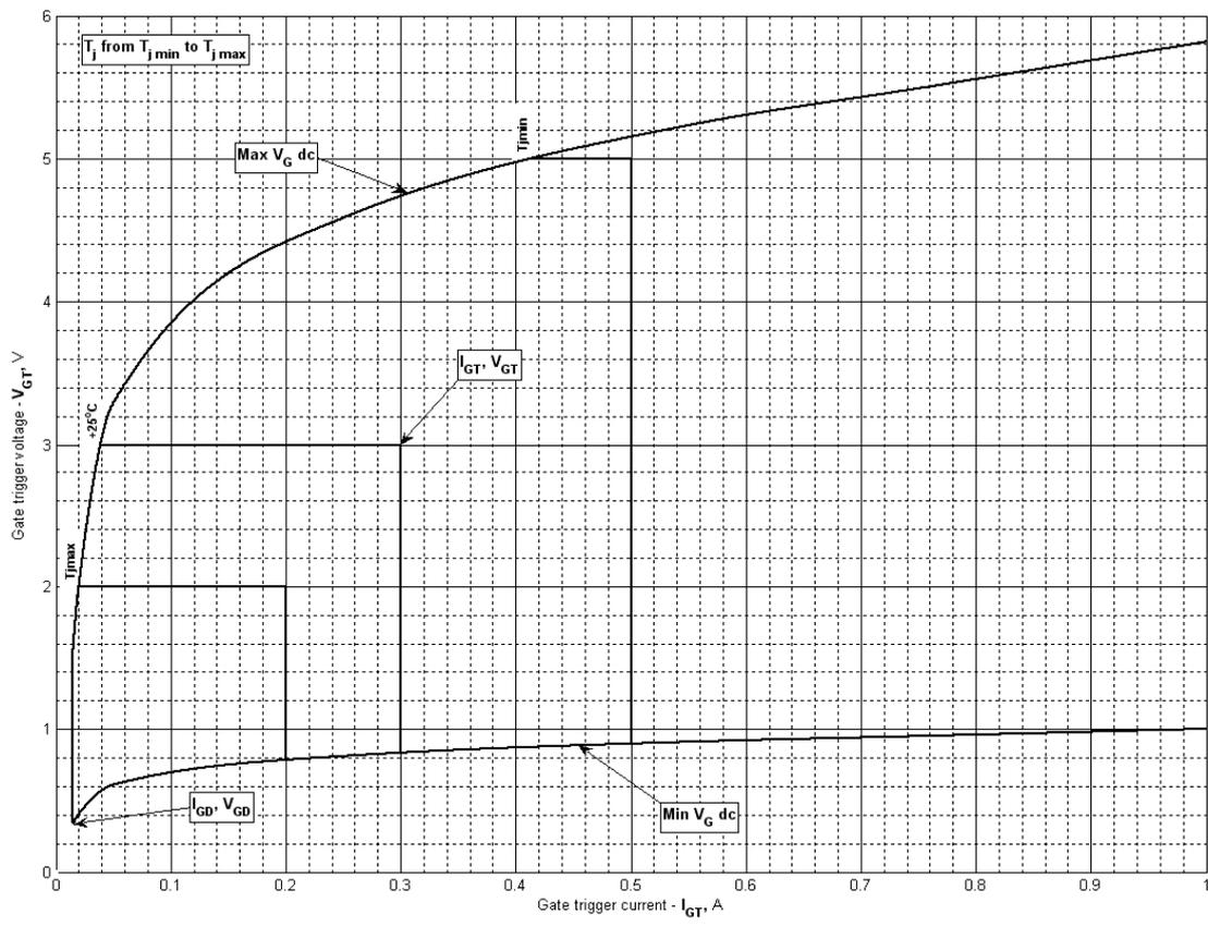
**Fig 3 – Gate characteristics – Trigger limits**
