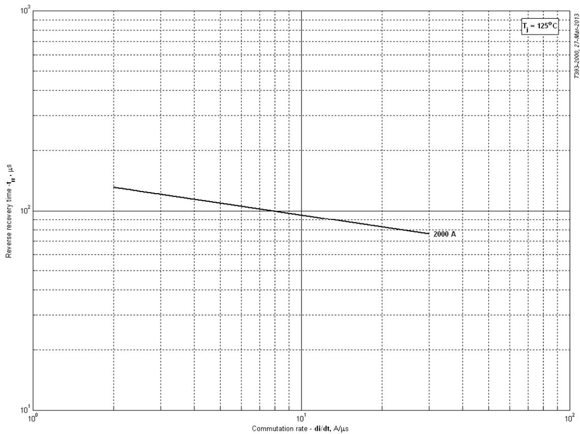
**Fig 8 – Maximum recovery time,  $t_{rr}$  (linear)**
