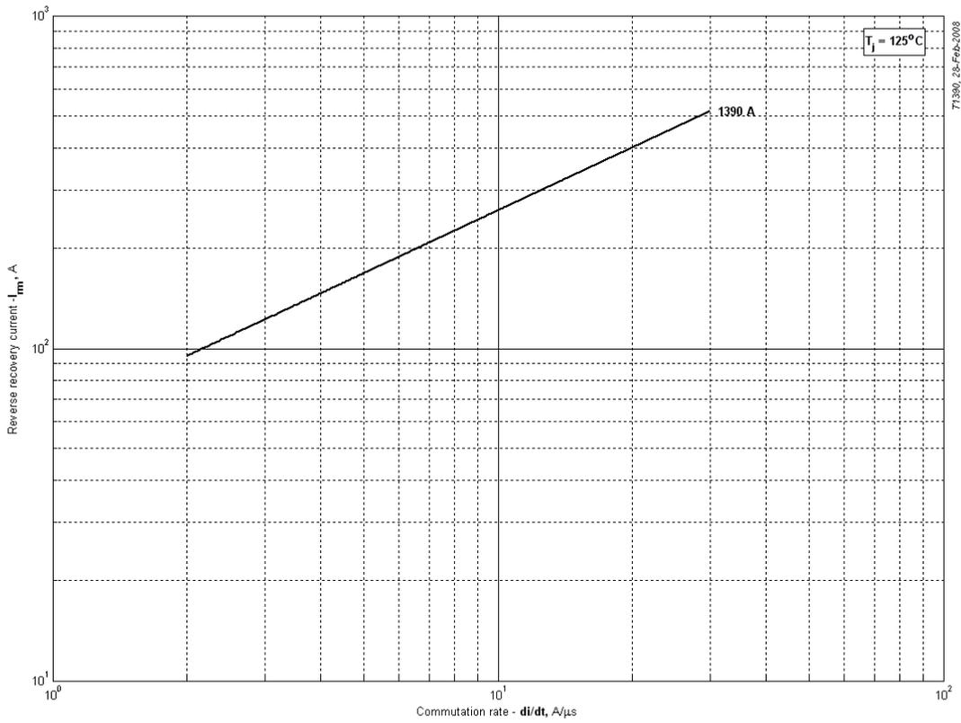
**Fig 7 – Peak reverse recovery current,  $I_{fm}$**
