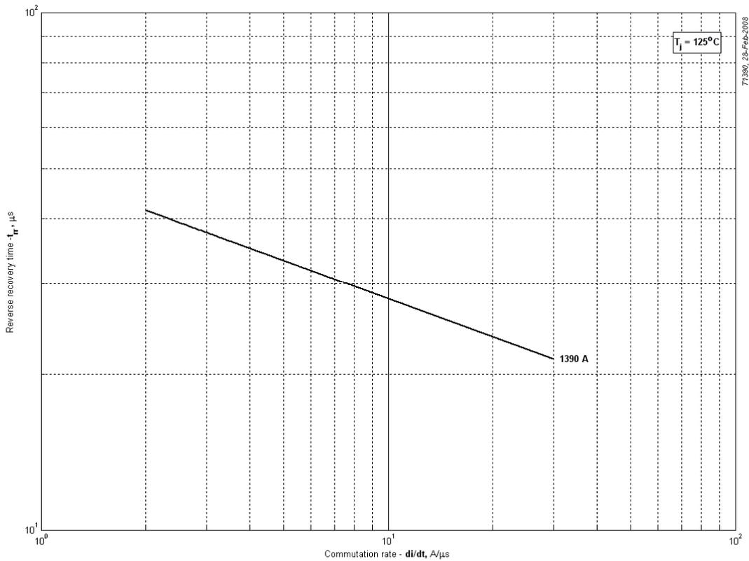
**Fig 8 – Maximum recovery time,  $t_{tr}$  (linear)**
