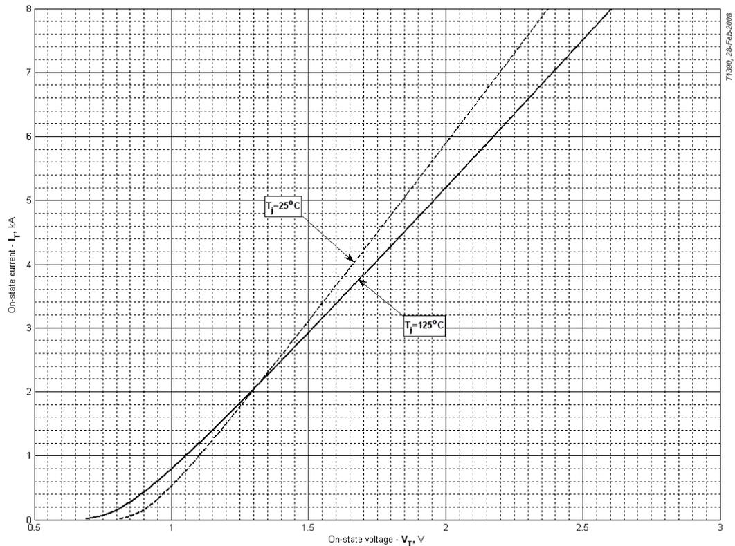
**Fig 1 – On-state characteristics of Limit device**
