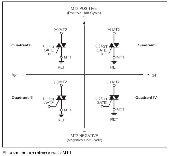
Whith in -phase signal (using standard AC lines) quadrants I and III are used
