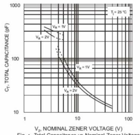
Fig. 4 Total Capacitance vs Nominal Zener Voltage
