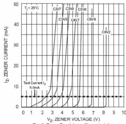
Fig. 2 Zener Breakdown Characteristics
