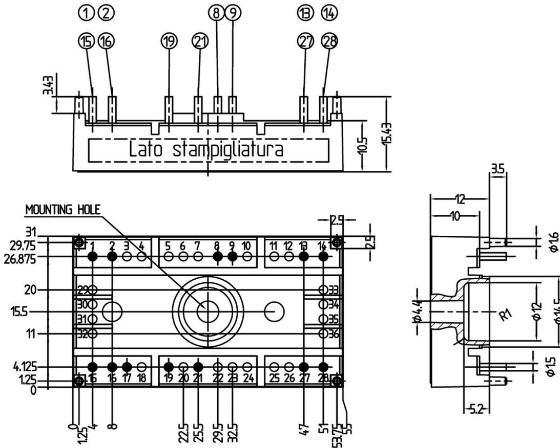
SUGGESTED HOLEDIAMETER FOR THE SOLDER PINS AND THE MOUNTING PINS IN THE PCB: 2 mm
