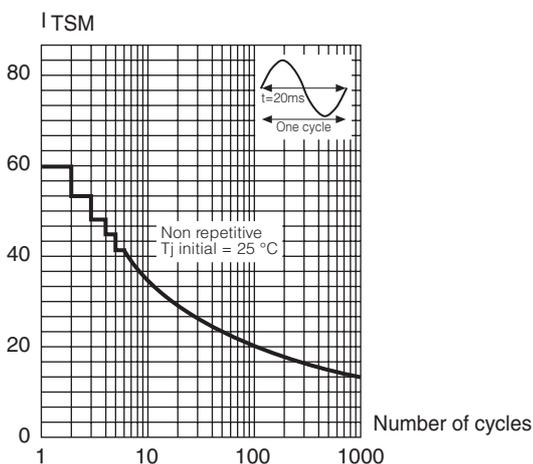
Fig. 6: Non repetitive surge peak on-state current for a sinusoidal pulse with width: tp < 10 ms, and corresponding value of I<sup>2</sup>t.
