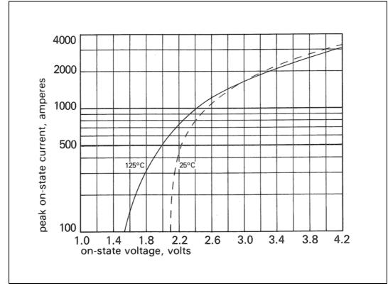
Figure 1 - On-state characteristics of Limit device
