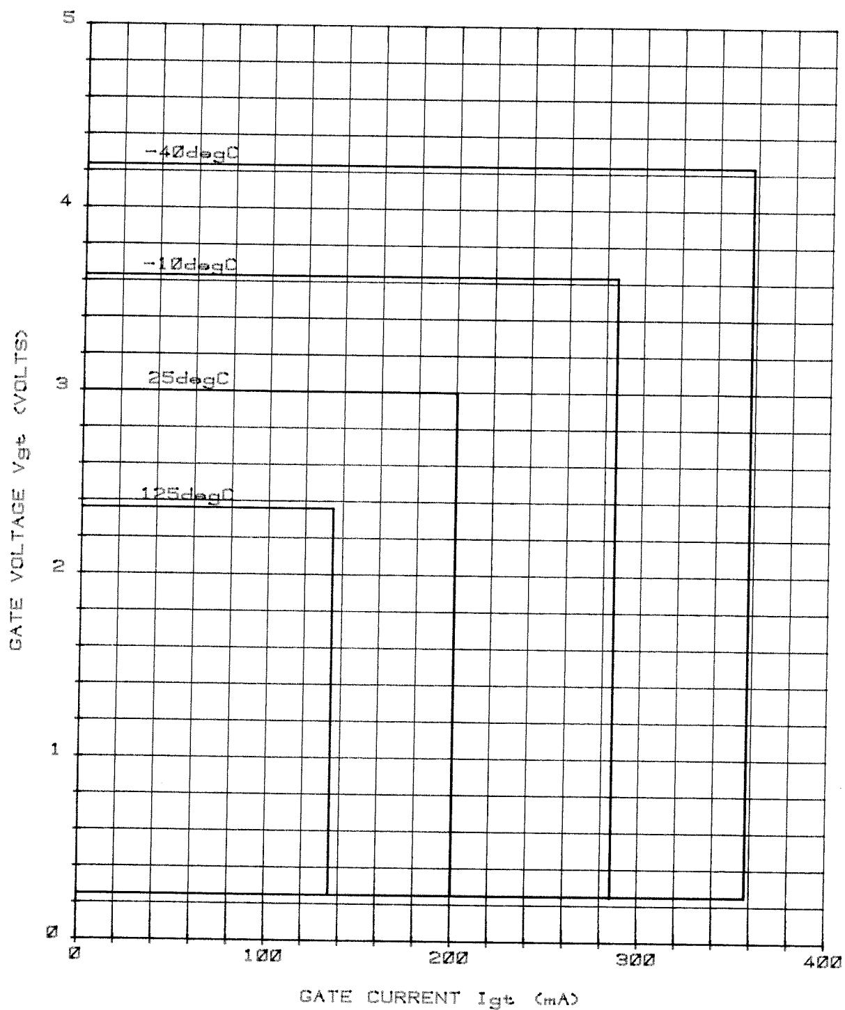
GATE CHARACTERISTICS AT 25°C JUNCTION TEMPERATURE
