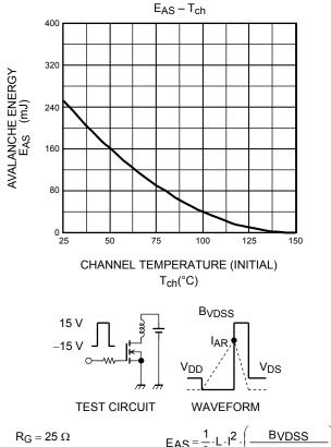
$$\begin{aligned} R_G &= 25~\Omega \\ V_{DD} &= 90~V,~L = 6.04~mH \end{aligned} \qquad E_{AS} &= \frac{1}{2} \cdot L \cdot I^2 \cdot \left( \frac{BVDSS}{BVDSS - VDD} \right) \end{aligned}$$
