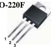
1.Gate 2. Drain 3. Source
