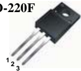
1.Gate 2. Drain 3. Source
