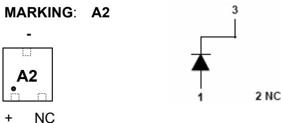
**Maximum Ratings and Electrical Characteristics, Single Diode @Ta=25°C**
