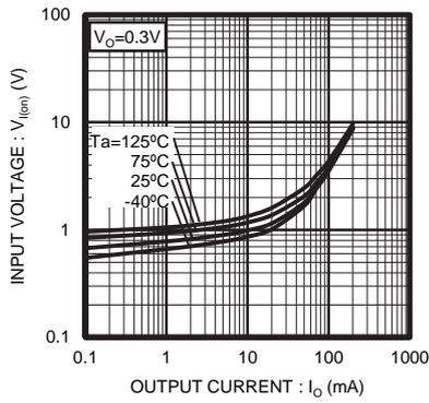
Fig 2. Input Voltage vs. Output Current (ON Characteristics)
