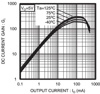
Fig 4. DC Current Gain vs. Output Current
