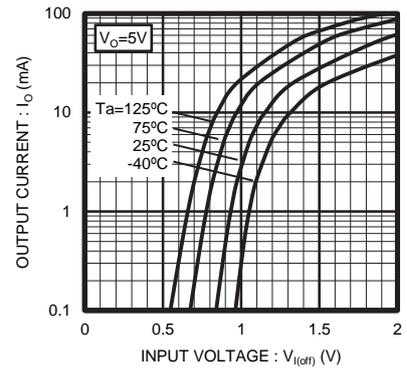
Fig 3. Output Current vs. Input Voltage (OFF Characteristics)
