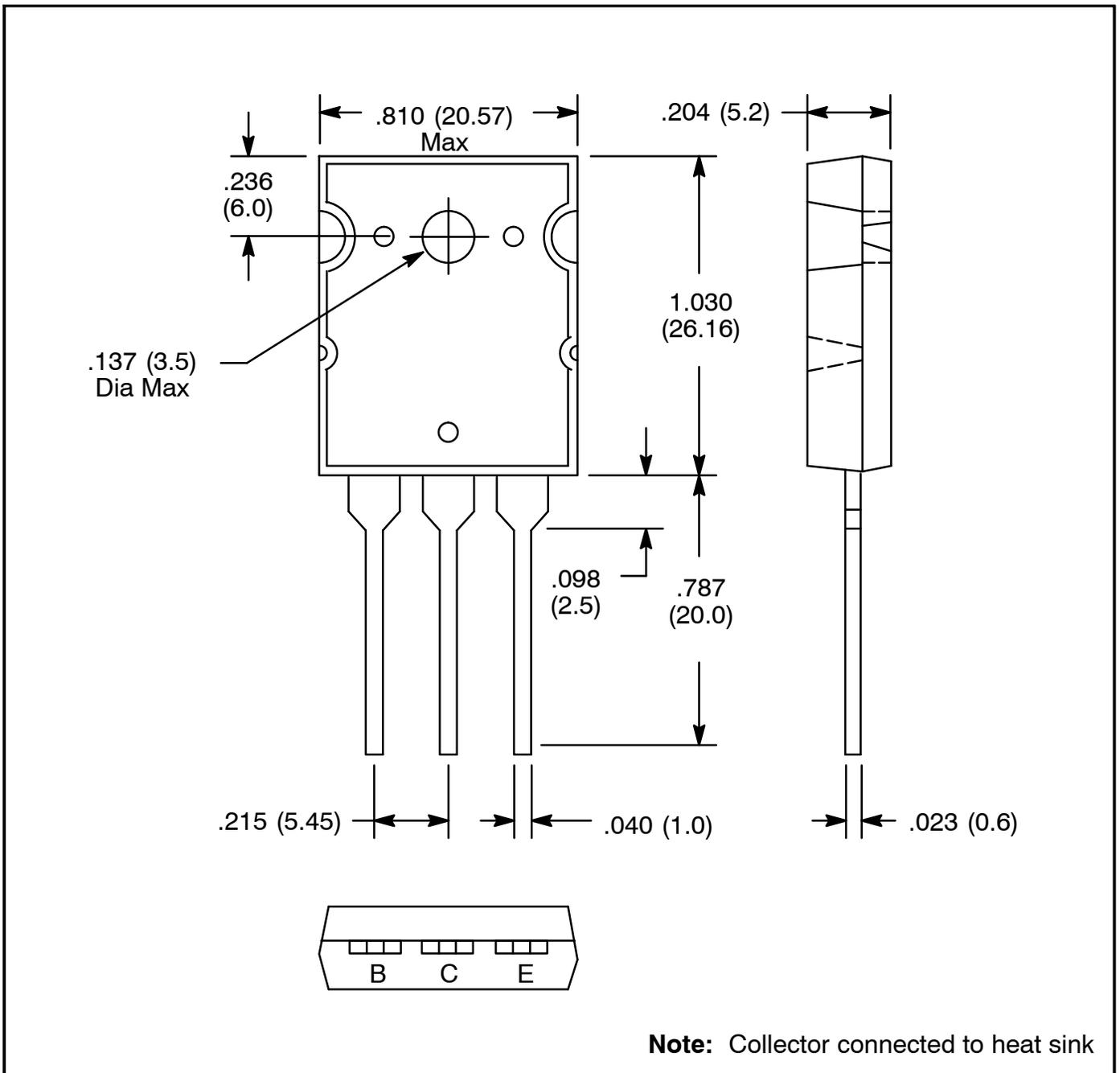
**Note:** Collector connected to heat sink
