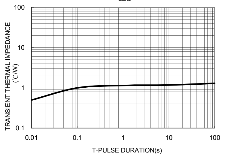
FIG. 6 TYPICAL TRANSIENT THERMAL IMPEDANCE PER LEG
