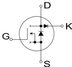
StarMOS is a new generation of high voltage N-Channel enhancement mode power MOSFETs. This new technology minimises the JFET effect, increases packing density and reduces the on-resistance. StarMOS also achieves faster switching speeds through optimised gate layout.
