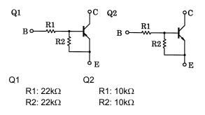
Q1: RN2403 Equivalent Q2: RN1402 Equivalent
