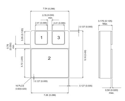
Bipolar NPN Device in a Hermetically sealed Ceramic Surface Mount Package for High
