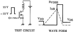
$$\begin{array}{l} \mathrm{R_{G}=25\ \Omega} \\ \mathrm{V_{DD}=25\ V,\ L=840\ \mu H} \end{array} \qquad \mathrm{EAS}=\frac{1}{2}\cdot\mathrm{L}\cdot\mathrm{I}^{2}\cdot\left(\frac{\mathrm{BVDSS}}{\mathrm{BVDSS}-\mathrm{VDD}}\right) \end{array}$$
