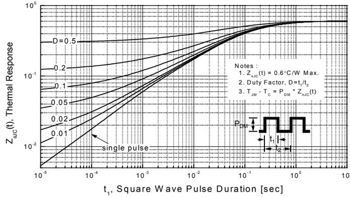
Figure 11-2. Transient Thermal Response Curve for FCPF20N60
