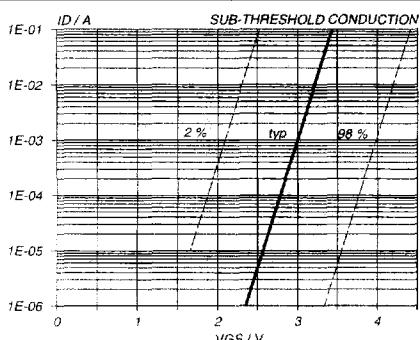
Fig.11. Sub-threshold drain current.
