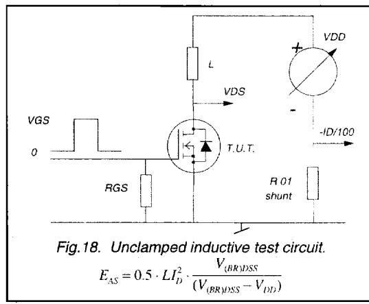
Fig. 18. Unclamped inductive test circuit.
