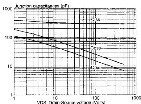
Fig.12. Typical capacitances,  $C_{iss}$ ,  $C_{oss}$ ,  $C_{rss}$ .
