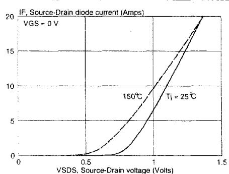
Fig.16. Source-Drain diode characteristic.
