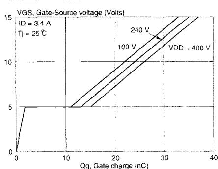
Fig.13. Typical turn-on gate-charge characteristics.
