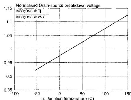
Fig.15. Normalised drain-source breakdown voltage.
