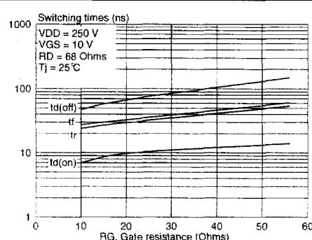
Fig.14. Typical switching times.
