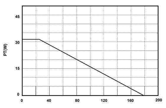
Power Dissipation(PT) vs. Case Temperature(Tc)
