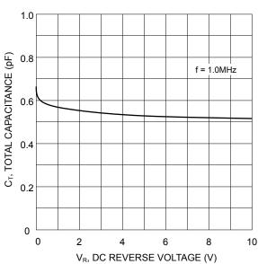
Fig. 3 Total Capacitance vs. Reverse Voltage
