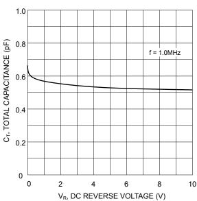
Fig. 3 Total Capacitance vs. Reverse Voltage
