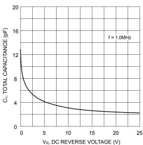
Fig. 3 Total Capacitance vs. Reverse Voltage
