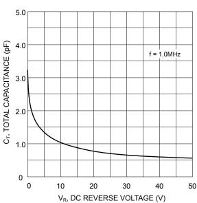
Fig. 3 Total Capacitance vs. Reverse Voltage
