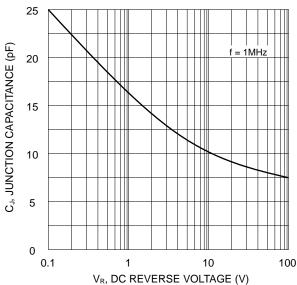
Fig. 5 Typical Junction Capacitance
