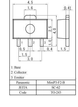
Note) \*1: Printed circuit board: Copper foil area of 1 cm $^2$  or more, and the board thickness of 1.7 mm for the collector portion Absolute maximum rating without heat sink for  $P_C$  is 0.5 W
