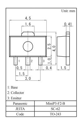
Note) \*1: Printed circuit board: Copper foil area of 1 cm<sup>2</sup> or more, and the board thickness of 1.7 mm for the collector portion
