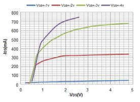
3. Dropout Voltage (V<sub>DS</sub>) Vs. Charge current (I<sub>DS</sub>), T = 25°C
