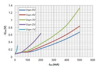
$6. \quad \ \ Dropout \ Voltage \ (V_{DS}) \ Vs. \ Charge \ current \ (I_{DS}),$
