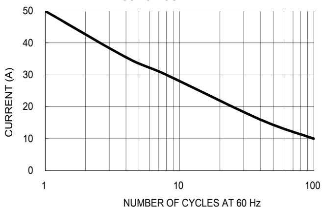
FIG. 2- MAXIMUM NON-REPETITIVE FORWARD SURGE CURRENT
